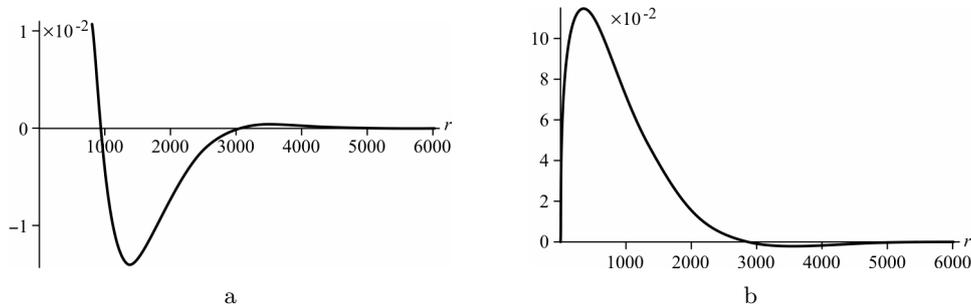
**Figure 3.** The dimensionless stress  $\tilde{\sigma}_{zz}$  as a function of radius at the frequency  $f = 2\text{Hz}$ : a) the real part, b) the imaginary part
