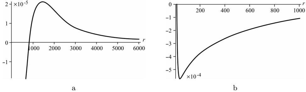
**Figure 1.** The dimensionless stress  $\tilde{\sigma}_{rr}$  as a function of radius at the frequency  $f = 2\text{Hz}$ : a) the real part, b) the imaginary part
