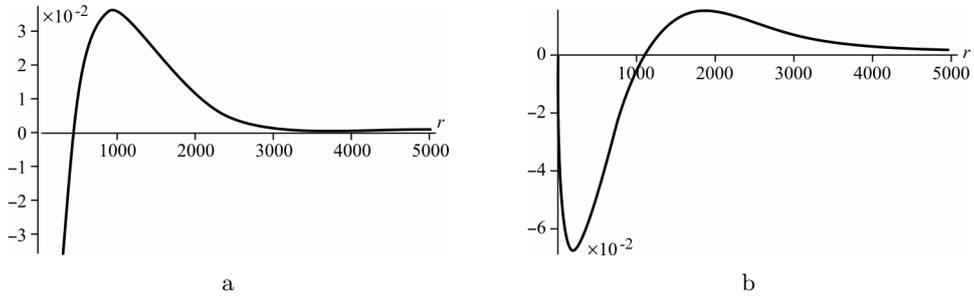
**Figure 2.** The dimensionless stress  $\tilde{\sigma}_{\theta\theta}$  as a function of radius at the frequency  $f = 2\text{Hz}$ : a) the real part, b) the imaginary part
